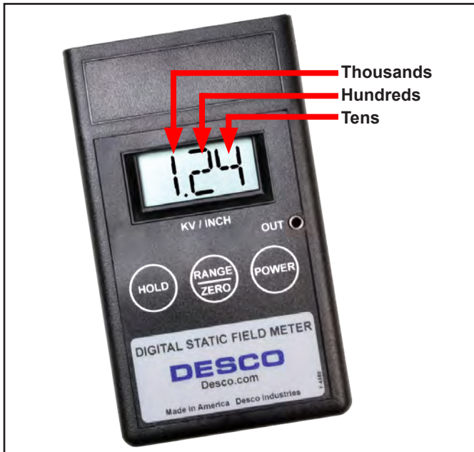
Figure 6. Reading the Digital Static Field Meter while in the \pm 20 kV range
