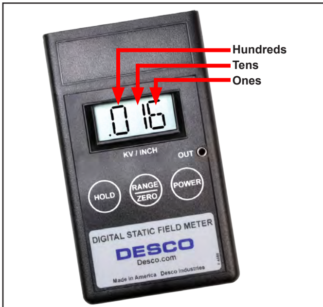
Figure 7. Reading the Digital Static Field Meter while in the \pm 2 kV range
